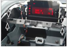
5. Remove the middle bar (cut at the position marked with arrows)
